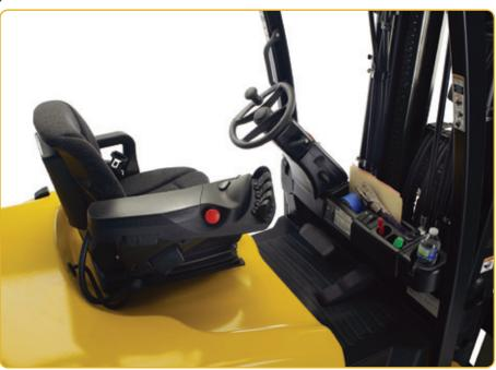
reducing fatigue and increasing productivity. A swivel seat option provides a superior reverse driving position.
