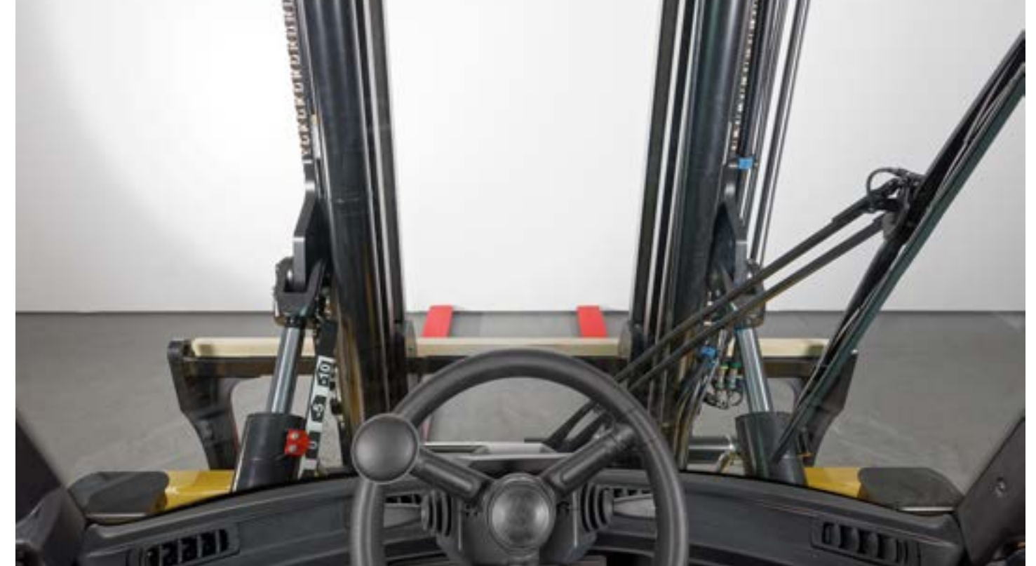
The operator has a clear view of the fork tips when in the operator seat
