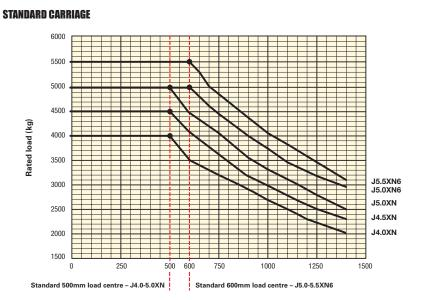
Load centre Distance from front of forks to centre of gravity of load.
