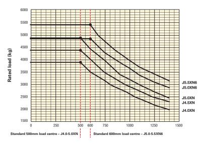
**NOTE:** Special forks with higher load ratings may be required to obtain full truck ratings with load centres 1400mm or greater.
